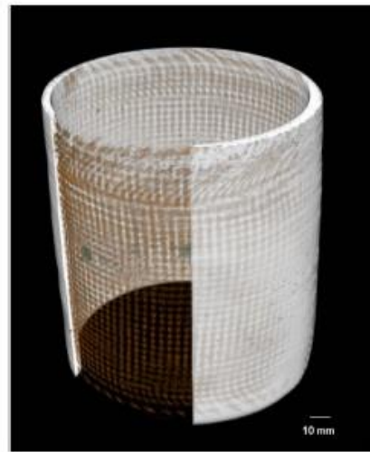
Fig. 9. Joint 4: 3D image demonstrating a small defect region in blue. (For interpretation of the references to colour in this figure legend, the reader is referred to the web version of this article.)
