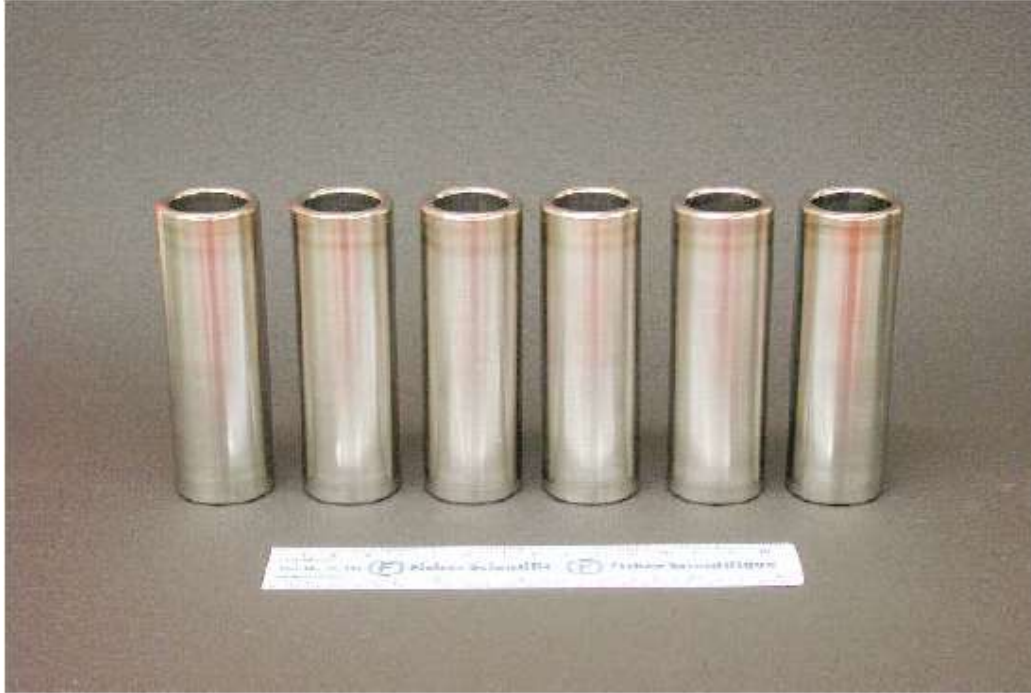
Figure 2-1: Six 10cm long annular specimens fabricated by AECL using VIPAC approach [4]
