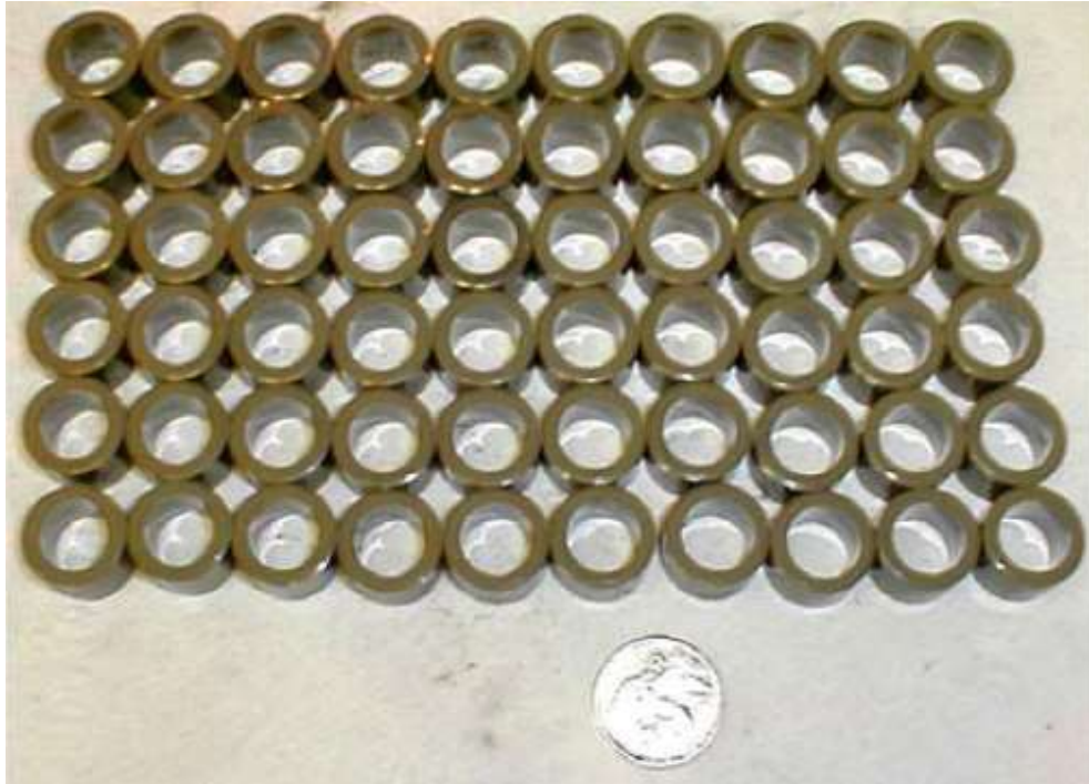
Figure 2-2: Annular pellets manufactured by Westinghouse using sintering process [4]
